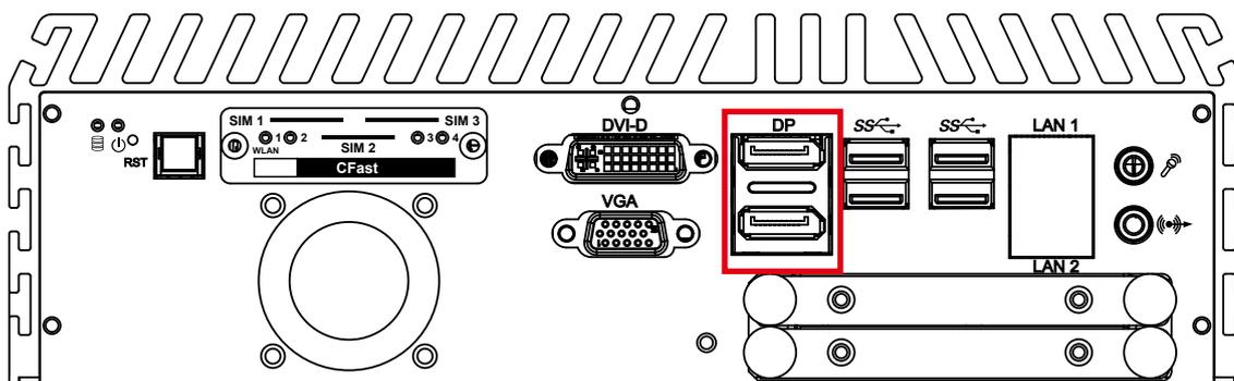
Onboard Display Port supports auxiliary channel dual mode and the connection supports up to 4096 x 2304 resolution at 60 Hz.
