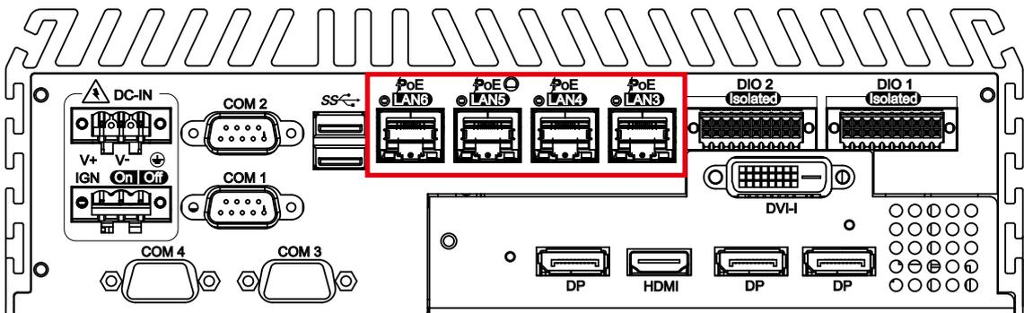
There are quad 8-pin PoE RJ-45 jacks supporting 10/ 100/1000 Mbps Ethernet connections in the front side. Powered by Intel I210 Ethernet engine. When both LAN 1 and LAN 2 work in normal status, iAMT 11.0 function is enabled. Each PoE supports 30.4W
