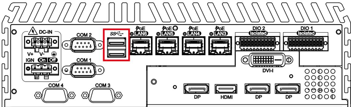
There are 2 USB 3.0 connections available supporting up to 5GB per second data rate in the front side of ECS-9700/9600 GTX950. It is also compliant with the requirements of Super Speed (SS), High Speed (HS), Full Speed (FS) and Low Speed (LS).
