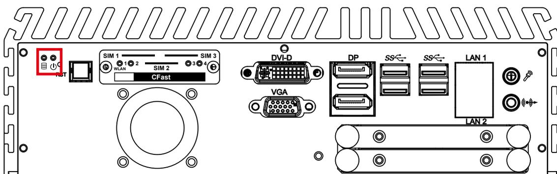
HDD LED/ Yellow : A Hard Disk/ CFAST LED. If the LED is on, it indicates that ECS-9700/9600 GTX950 storage is functional. If it is off, it indicates that the system's storage is not functional. If it is flashing, it indicates data access activities.
