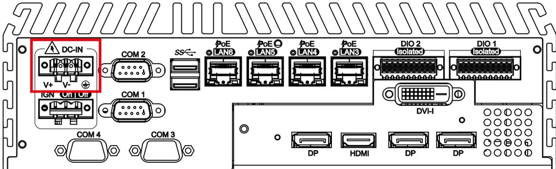
This system supports 10V to 36V DC power input by terminal block in the rear side. In normal power operation, power LED lightens in solid green and supports up to 80V surge protection.
