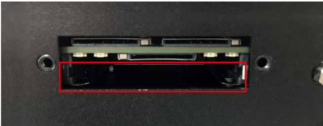
**Step 4** Insert CFast card and push to lock.
