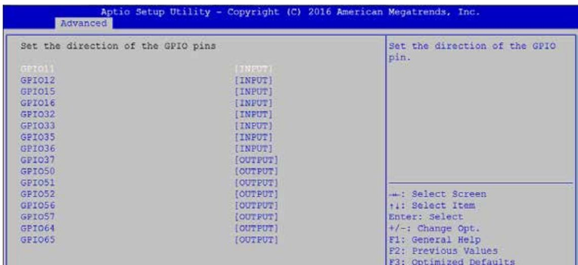
Figure 4-3-6-3: GPIO Pin Input/Output Settings of SIO IT8786
