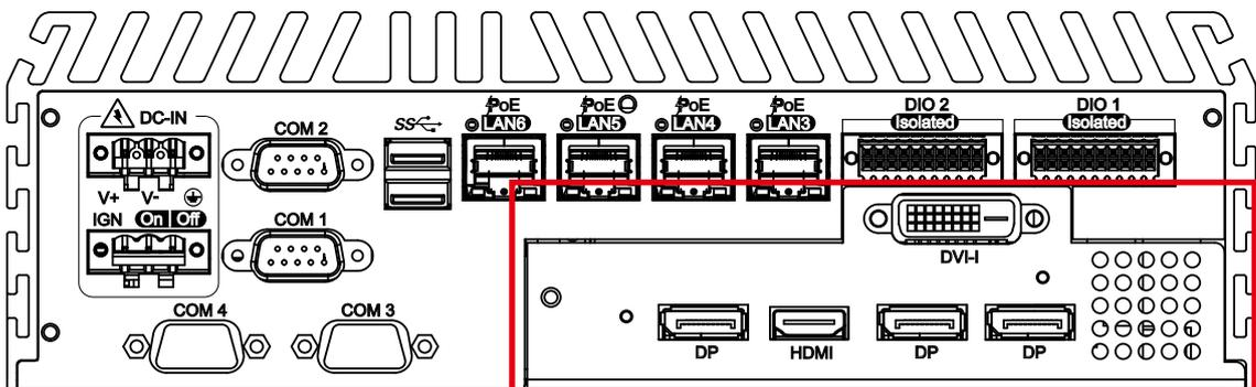
You could have 4 independent displays as your wish from these 5 display ports. Also, you could have four 4K resolution displays, the 3 DisplayPort and a HDMI, from these 5 ports.
