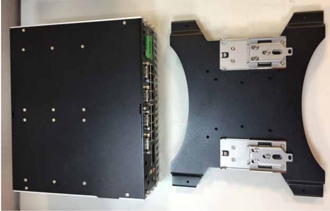
**Step 2** Take ECS-9700/9600 GTX950 and Din Rail Kit and fasten four KHS#6-32 screws in the four marked corners.
