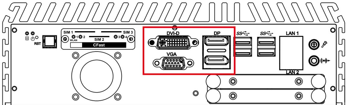
You could have 3 independent displays as your wish from these 4 display ports. Also, you could have two 4K resolution displays, the 2 DisplayPort, from these 4 ports.
