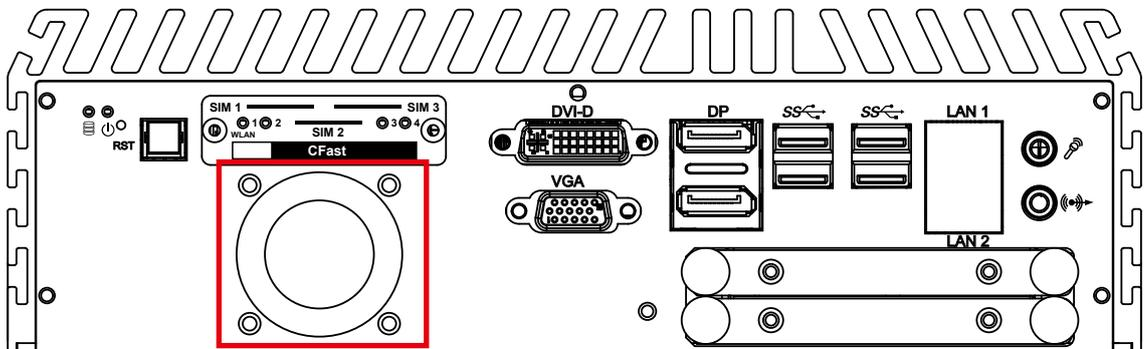
There is a system FAN on front side for airflow direction outward. You can adjust the FAN Speed from Vecow BIOS Setting. (refer to 4.3.7\_Hardware Monitor\_FAN PWM Value)
