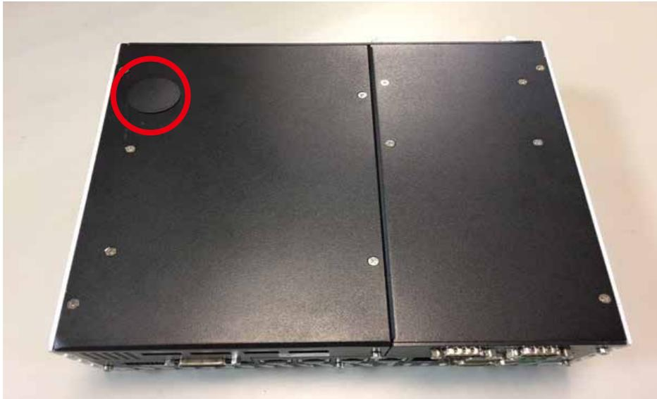
**Step 2** Remove two F#6-32 screws (circled in red) and two F-M3 screws (circled in yellow) on the bottom side.
