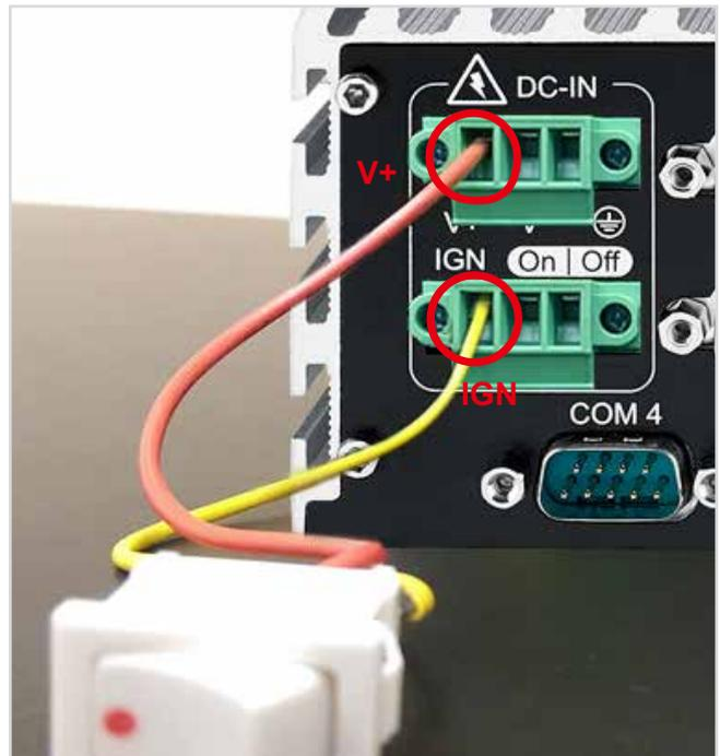
For testing purpose, you can refer to the picture above to simulate ignition signal input controlled by a latching switch.
