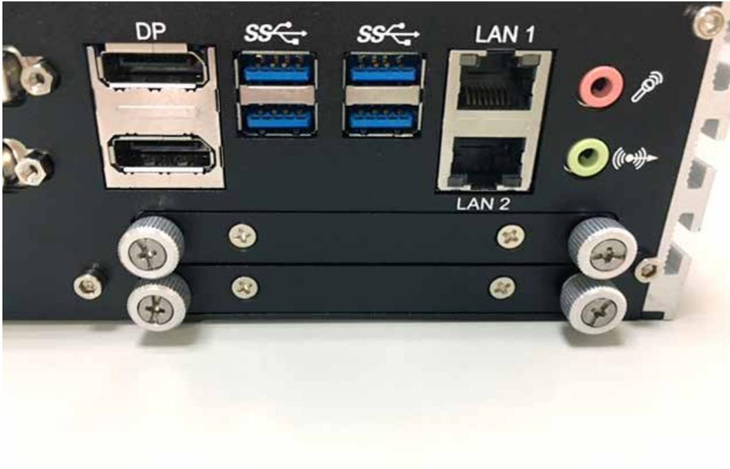
**Step 2** Insert 2.5" SSD/HDD in the tray and fasten two F-M3x4 screws.
