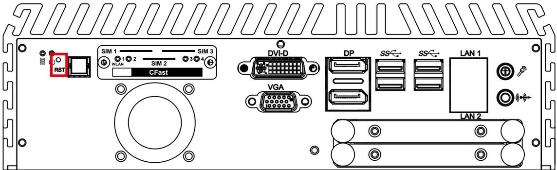
It is a hardware reset switch. Please use this switch to reset ECS-9700/9600 GTX950 without power off. Press the Reset Switch for a few seconds, and then reset will be enabled.
