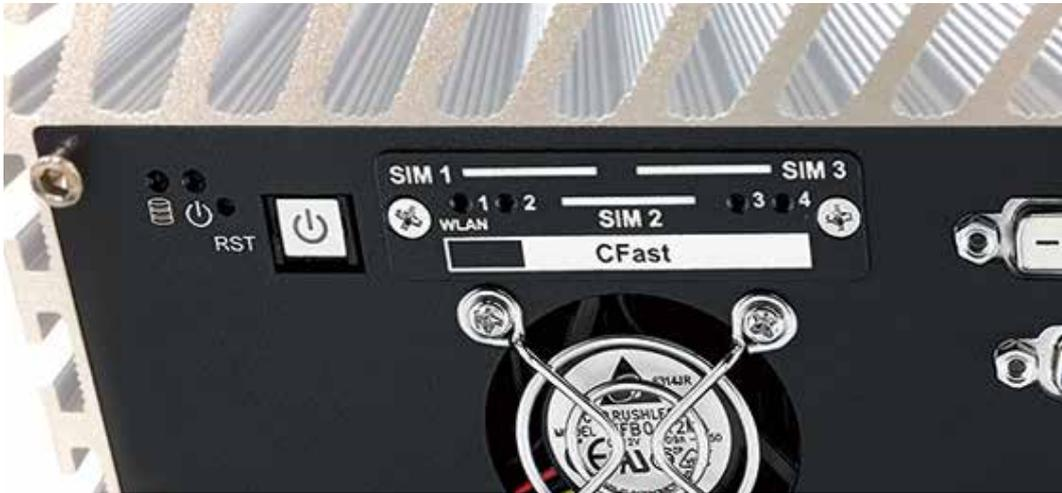
**Step 2** Before Inserting CFast & SIM Card, make sure ECS-9700/9600 GTX950 power is not plugged.
