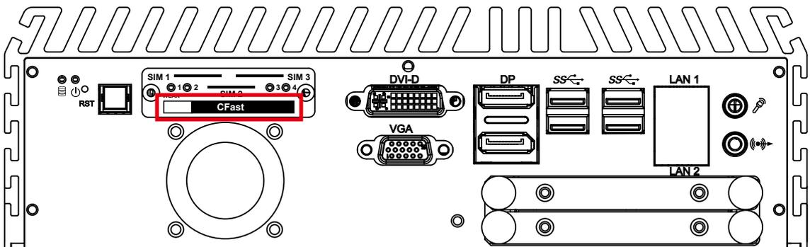
There is a CFast socket on the front panel supporting Type-I/II Compact Flash card. It is implemented by a SATA III Port from CM236 PCH. Be sure to disconnect the power source and unscrew the CFast socket cover before installing a CFast card. The ECS-9700 does not support the CFast hot swap and PnP (Plug and Play) functions. It is necessary to remove power source first before inserting or removing the CFast card.
