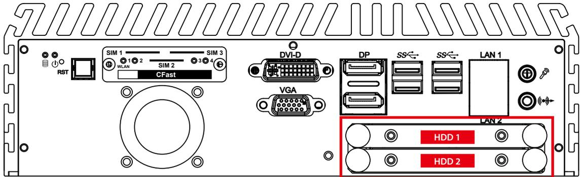
There are 2 front-access 2.5" SSD/ HDD trays in the front side of ECS-9700/9600 GTX950. Just trigger to open the SSD/ HDD tray, up to 8TB is available.
