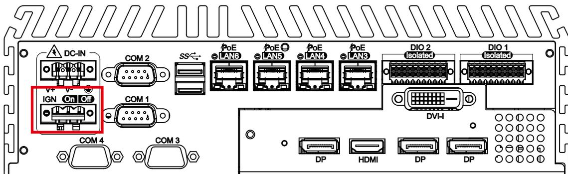
It is a 5-pin power-on or power-off switch through Phoenix Contact terminal block. You could turn on or off the system power by using this contact. This terminal block supports dual function of soft power-on/ power-off (instant off or delay 4 second), and suspend mode.
