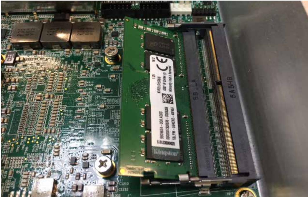
**Step 2** Make sure the RAM module is locked by the memory slot.
