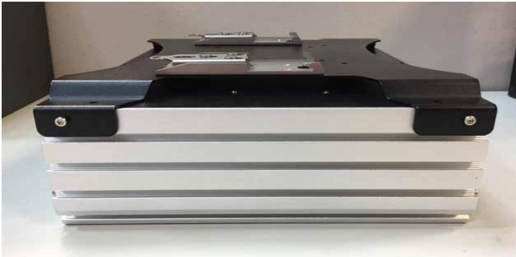
**Step 5** ECS-9700/9600 GTX950 With Din Rail.
