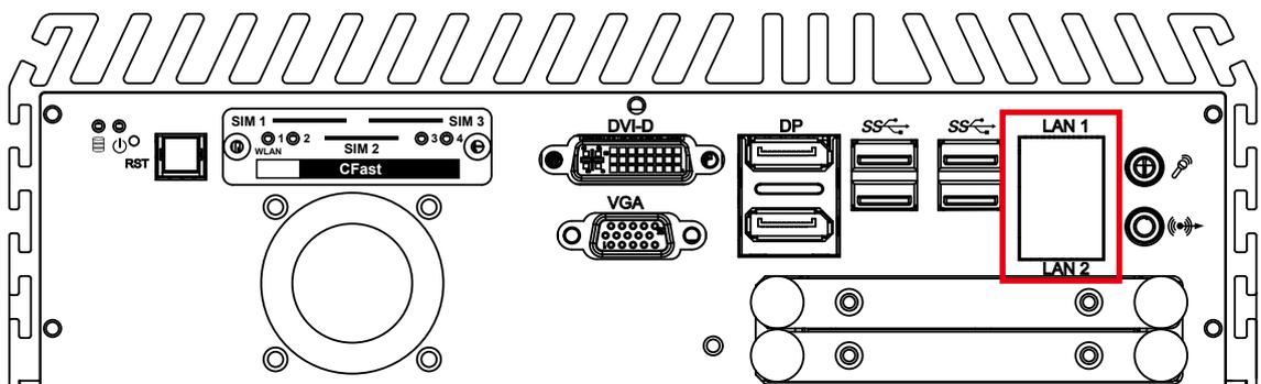
There are dual 8-pin RJ-45 jacks supporting 10/ 100/1000 Mbps Ethernet connections in the front side. LAN 1 is powered by Intel I219 Ethernet Phy and LAN 2 is powered by Intel I210 Ethernet engine. When both LAN 1 and LAN
