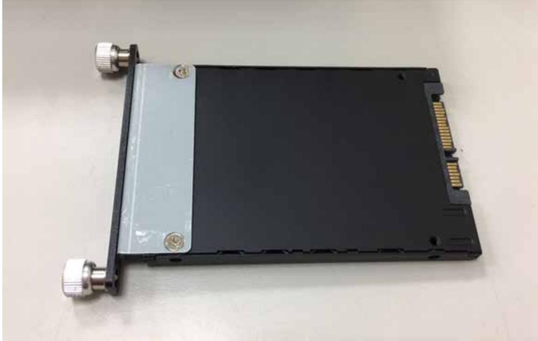
**Step 4** Installing SSD/HDD.
