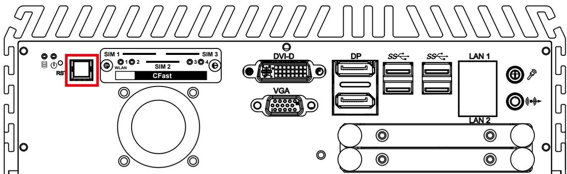
The Power Button is a non-latched switch with dual color LED indications. It indicates power status: S0, S3 and S5. More detail LED indications are listed as follows:
