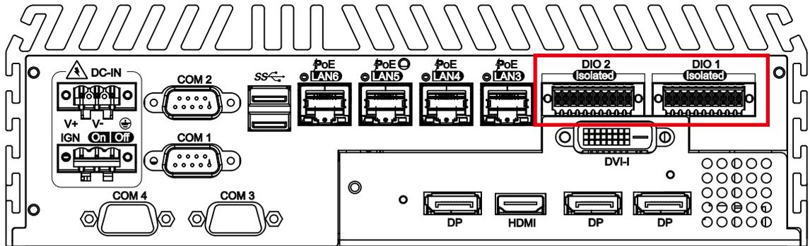
There is a 32-bit (16-bit DI, 16-bit DO) with 2 DIO connectors in the rear side. DI/DIO supports NPN(sink) and PNP(Source) mode, and each DI channel is equipped with a photocoupler for isolated protection. Each DO with isolator chip is configured by a Jumper for each DIO connector.
