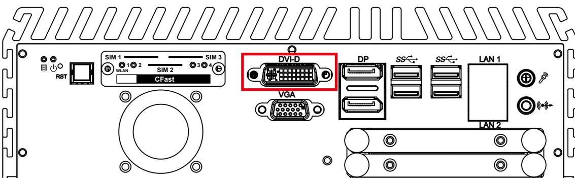
The DVI-D connector on the front panel supports DVI display. This connector can output DVI signal. The DVI output mode supports up to 1920 x 1200 resolution and the DVI is automatically selected according to the display device connected. You will need a DVI-D cable when connecting to a display device.
