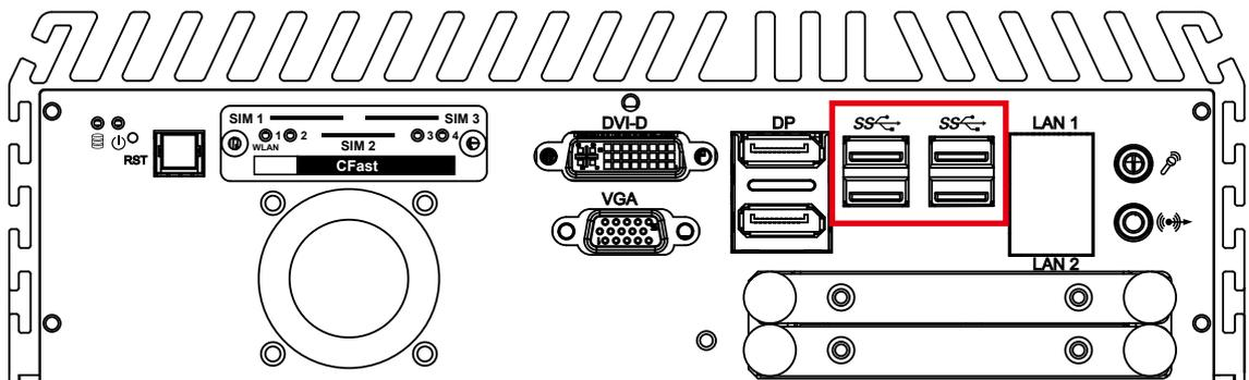
There are 4 USB 3.0 connections available supporting up to 5GB per second data rate in the front side of ECS-9700/9600 GTX950. It is also compliant with the requirements of Super Speed (SS), High Speed (HS), Full Speed (FS) and Low Speed (LS).
